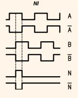
Pulse trains: Clockwise rotation when looking at the end of the shaft. (mounting side)
